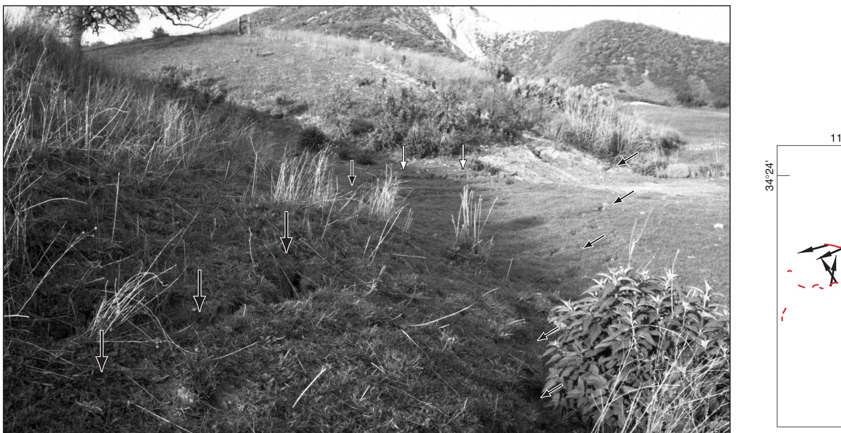
Figure 2. Broad zone of surface fractures, located between vertical and diagonal arrows, on north side of Potrero Canyon. Fractures below vertical white arrows in midground show stair-step pattern indicative of valley fill, located to right, that moved away from bedrock. View to the northeast.
