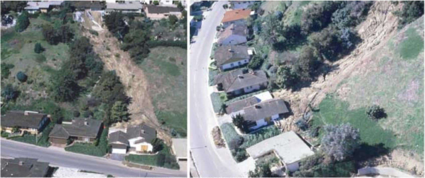
Figure 2 Debris flow, Monterey Park, Los Angeles County, 1980. Debris flow is in Pleistocene alluvial deposits.
