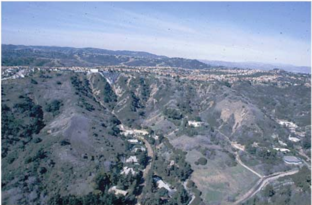
Figure 28 Santa Monica Mountains, Los Angeles County, 1980. View is to the west. More debris flows occurred on south facing slopes than on north facing slopes. Note the difference in vegetation between the north-and south-facing slopes.
