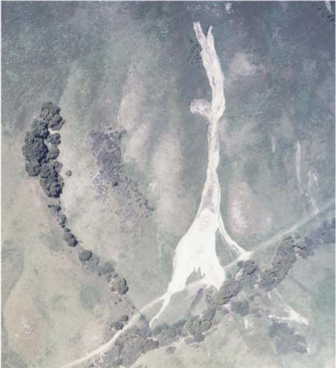
Figure 20 Relatively large disintegrated debris flow deposited on hillside, Las Cruces area, Santa Barbara County, 2001. Note road for scale.
